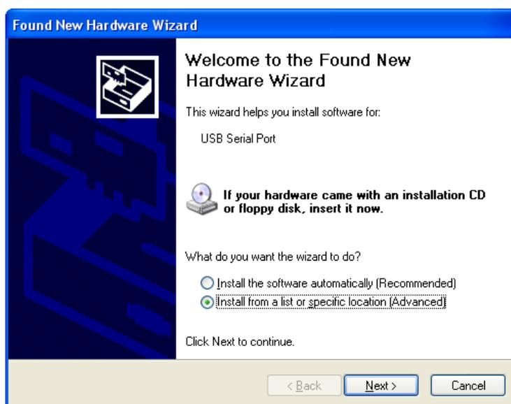
7. Windows will now install software for the newly created USB Serial Port. Select **'Install from a list or specific location (Advanced)'**.
